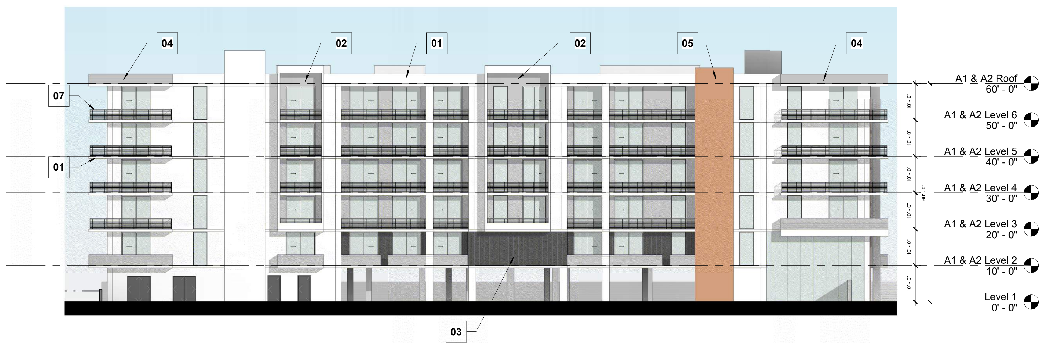
3 BLDG A2 - SOUTH ELEVATION A3.02 SCALE: 1/16" = 1'-0"
