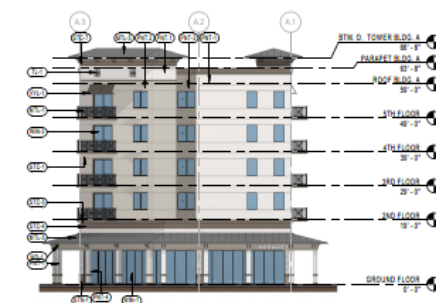
4 BUILDING A - SOUTH ELEVATION 1/16" = 1'-0"
