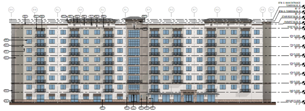
1 BUILDING B - NORTH ELEVATION 1/8" = 1'-0"
