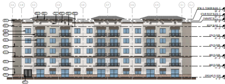
2 BUILDING C - SOUTH ELEVATION 1/8" = 1'-0"
