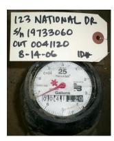
NMS' proposal can include provisions for exit testing of all replaced meters during this project. Certified meter test data will be provided to the Utility in an electronic format.
